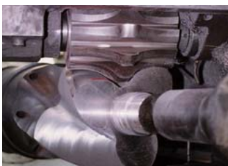
● Rotor processing using a milling machine
